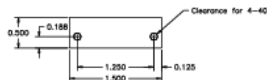
Part 21-004, Alignment Jig (for linear stage). Aluminum. (1 reqd)
