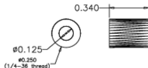
Part 21-019, Threaded Attachment for Fibers, Type 2. Make by modifying part provided. (1 reqd)
