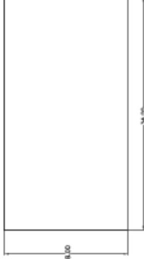
Part 12-036, Back/door Sheathing for computer box. (2 reqd)
