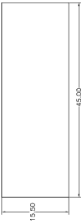
Part 12-017, Back/Door Sheathing for electronics box. (2 reqd)
