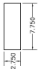
Part 10-022, Front Bumper/Tie Plate of Altitude Drive Attachment. Make of 1-in aluminum plate. (1 reqd)
